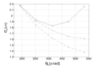
Figure 2: Horizontal beam size vs angular divergence at the SLC IP showing the reduction in beam size for larger  $\theta^*$ . The upper curves are for the 1996 optics, calculated using the RMS beam size (solid) and correct luminosity-weighted effective beam size (dashed). The lower curve (dot-dashed) is for the 1998 optics.
