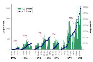
Figure 1: SLD luminosity showing the performance improvement from 1992-1998. The bars show luminosity delivered per week and the lines show integrated luminosity for each run. The numbers give average polarization.
