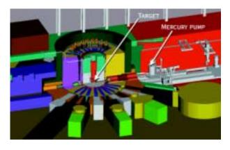
Figure 1: Cross-sectional view of the bulk shielding, shutters, instruments, maintenance cells, and mercury target.
