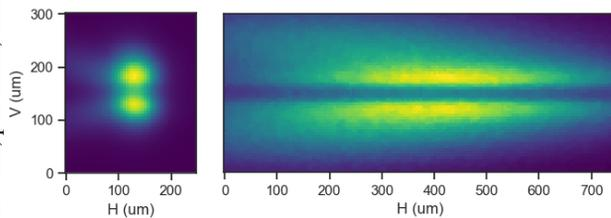
Figure 5: An optimally resolved  $\pi$  mode image in low-emittance (left) and nonlinear optics (right) configurations.
