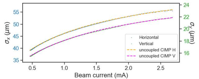
Figure 3: Dependence of  $1\sigma$  beam sizes on current for near-round beam, in minimally coupled lattice.
