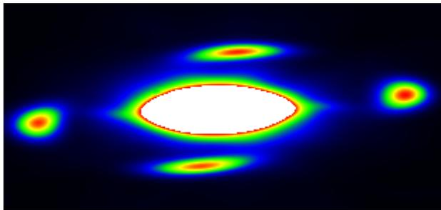
Figure 6: Transverse beam profile after injection near 1/4 resonance with nonlinear octupole insert on. Black denotes no signal, and white a complete saturation.
