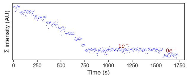
Figure 4: Post-processed sum of pixel intensities for a single camera, showing discrete steps as electrons are lost.
