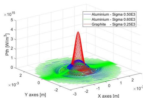
Figure 2: Thermal power distribution on the OTR hotspot.
