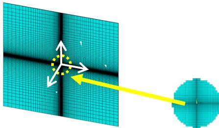
Figure 1: OTR screen finite element model.
