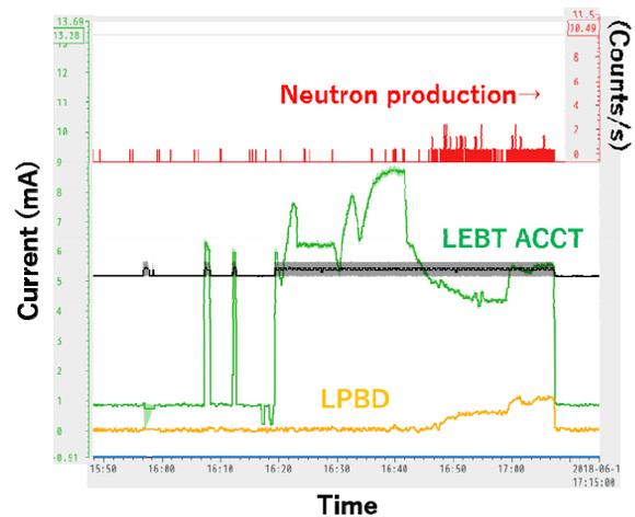
Figure 3: Beam current and neutron production trends when the beam reached to LPBD first time.
