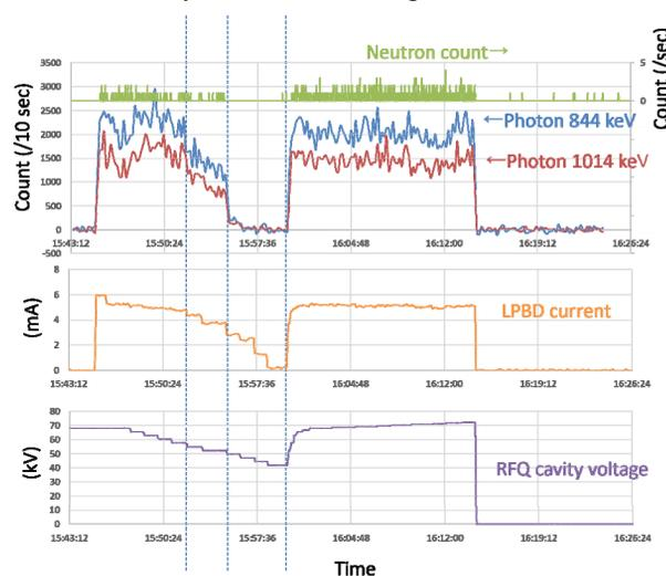
Figure 5: Relationship between the neutron/gamma count rates and the LPBD current and the RFQ cavity voltage.
