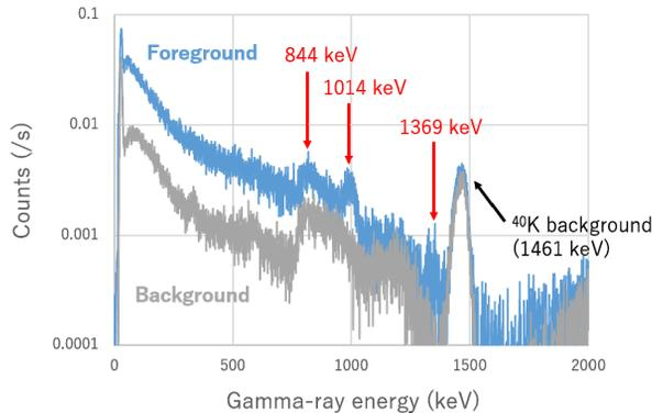
Figure 4: Gamma-ray spectrum observed at LPBD with  $\text{LaBr}_3(\text{Ce})$  detector in the day-1 experiment.
