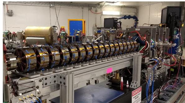
Figure 2: IOTA octupole insert in segment B2L. RF cavity and synchrotron radiation diagnostics in the background.
