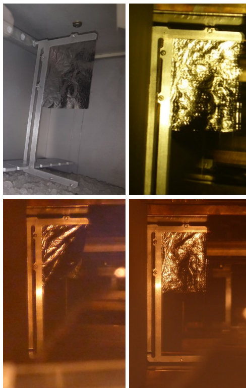
Figure 2: The first annealed DLC foil used – clockwise from top left: before installation, after 2.9 mAh, 17 mAh, and on removal after 136 mAh.
