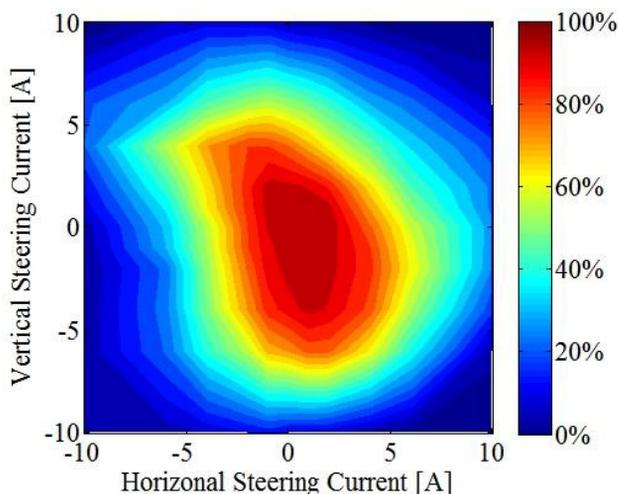
Figure 5: Proportion of the beam from T4 reaching FDC2 when sweeping the solenoid 1 integrated steering dipoles.
