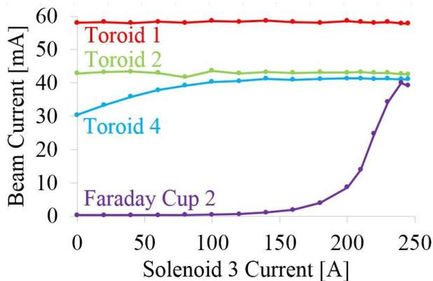
Figure 4: Measured beam current throughout the LEBT, as a function of solenoid 3 current. Solenoid 1 current fixed at 140 A. Faraday cup 1 and toroid 3 measurements were identical to toroid 2, so are omitted for clarity.
