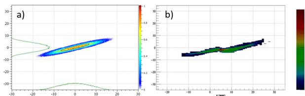
Figure 2: 7 mA proton beam distribution in phase space at the low energy beam transfer line emittance meter position (between the two LEBT solenoids). a) simulated distribution in phase-space, with the same set of solenoid strength b) Measured distribution in phase-space with the same set of solenoid couples. The simulated normalized rms emittance is 0.075 mm mrad, while the measured one is 0.08 mm mrad.
