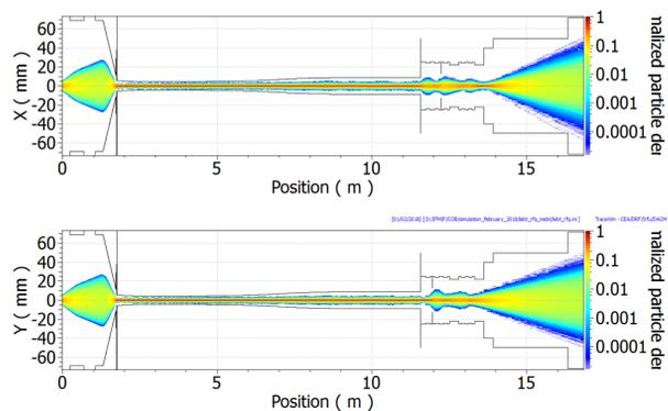
Figure 3: Macroparticle densities with respect the beam axis, starting outside the extraction column and up to the LPBD.
