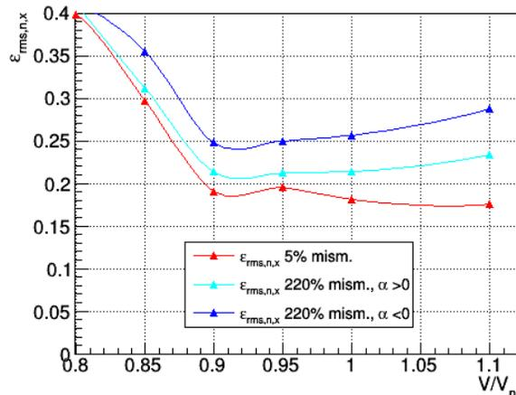
Figure 5: Transverse emittances measured at the end of the MEBT for different RFQ input mismatches.
