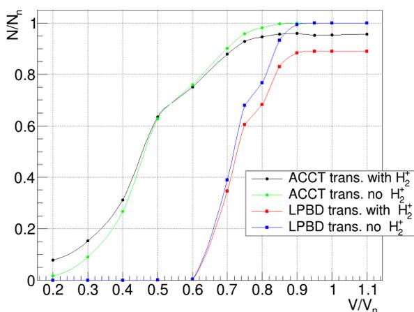
Figure 6: Proton transmission from the RFQ with respect different voltage ratios at the MEBT ACCT and the LPBD. The two curve ensembles are related to the calculations with and without contaminants.
