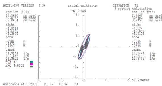
Figure 1: Output at 20 cm from the plasma electrode aperture for 13 mA proton beam.
