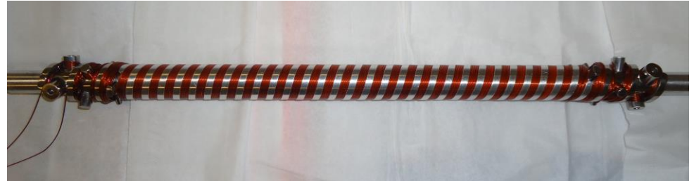
Wound 300-mm long prototype core.
