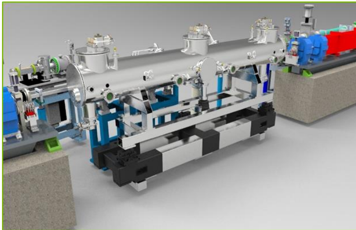
Design model of long SCU installed in the APS-U.
