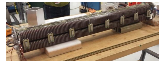
Photograph of 1.1-m long SCU magnet.
