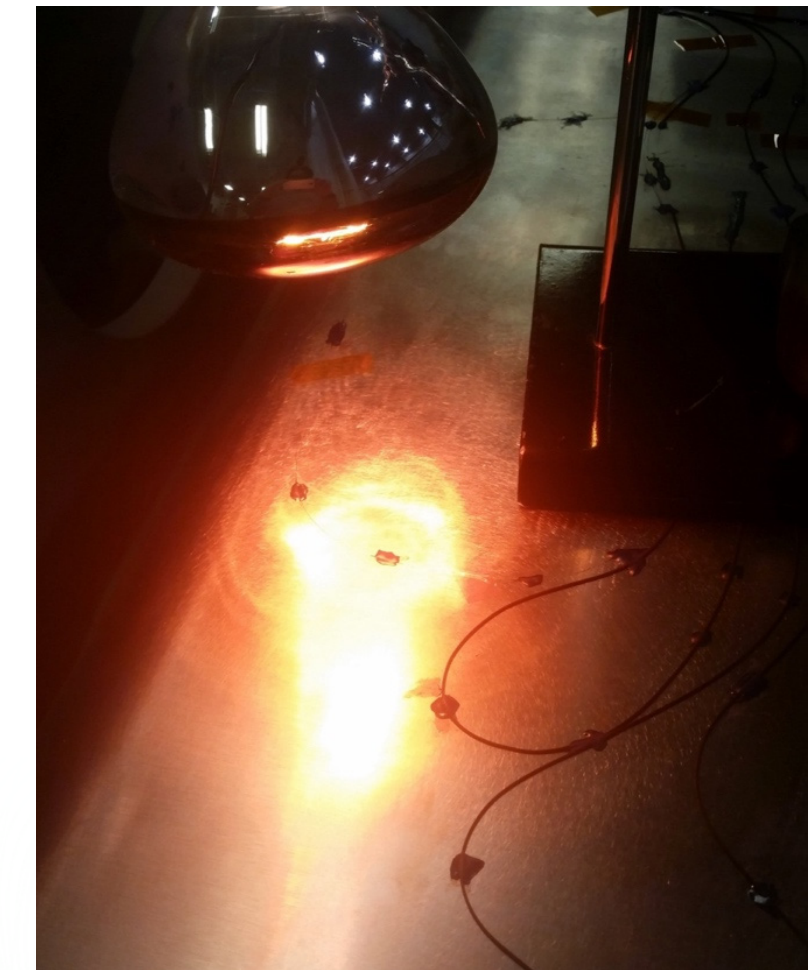
Curing of epoxy
