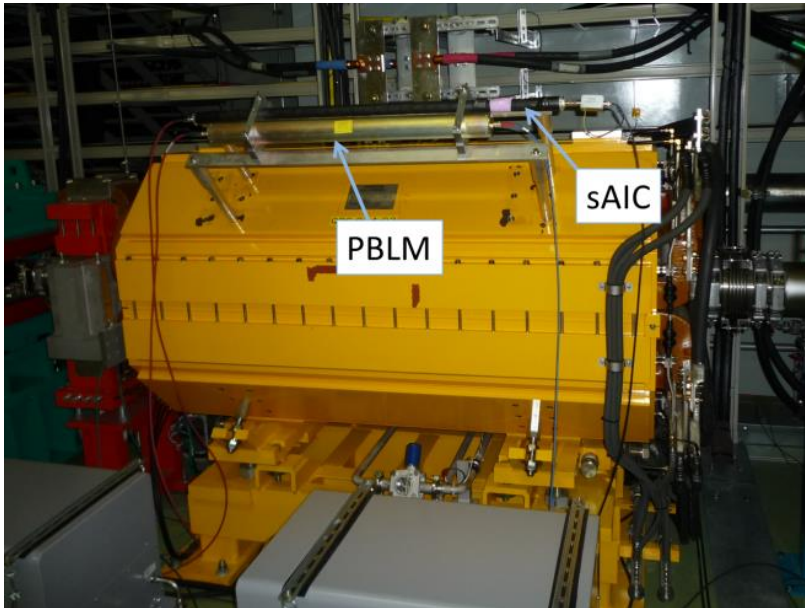
PBLM and sAIC installed at QM 848 mm from the beam line
