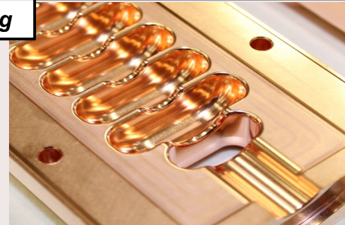
Novel split-block assembly for novel gap accelerator
