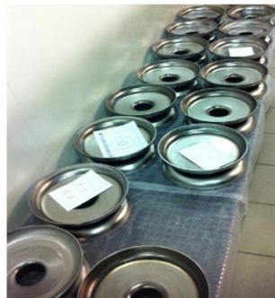
Dumbbells after welding in the control area
