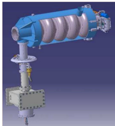
Spoke & Elliptical cavity package
