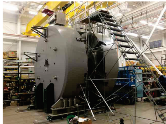
Figure 2. The MSU cyclotron gas-stopper magnet with the iron yoke open and the two coil cryostats installed in the iron pole pieces. The magnet height is ~5 meters.
