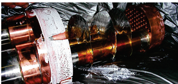
Figure 1: Drop-in cooler with a 2 nd -stage condenser [7].
