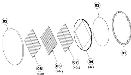
Figure 7: Ir, TZM and CuCrZr specimens in high-Z capsule.
