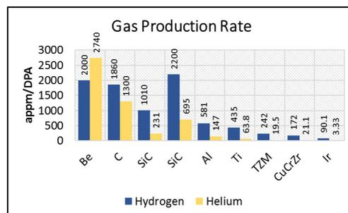
Figure 10: Peak gas production rate in the BLIP materials.
