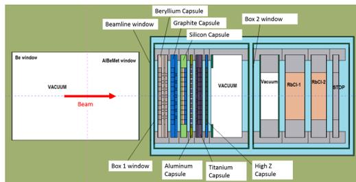
Figure 1: Targets arrangement in BLIP beam line.
