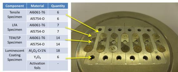
Figure 5: Aluminum capsule with various specimen types.
