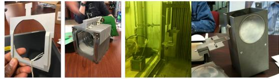
Figure 8: BLIP capsule holders, target basket and target box.
