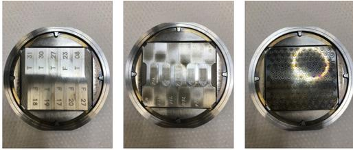
Figure 6: Titanium capsule showing fatigue (left), tensile and microstructural (middle), and meso-scale fatigue (right) specimens.
