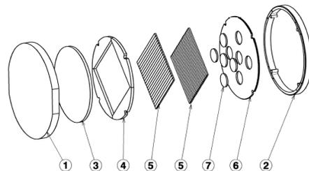
Figure 4: Silicon capsule with Si and SiC-coated graphite specimens.
