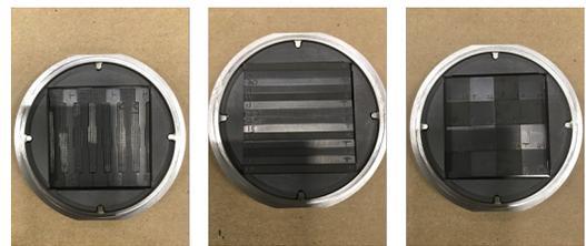
Figure 3: Graphite capsule showing tensile and CTE (left), bend (middle), and HiRadMat (right) specimens.
