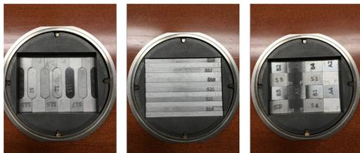
Figure 2: Beryllium capsule showing tensile and microstructural (left), bend (middle), and HiRadMat (right) specimens.
