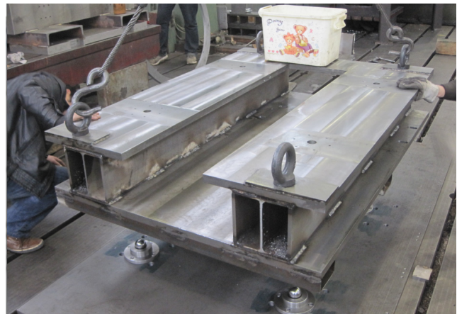
Figure 9: Support system of primary collimator with four balls and four pair ball-sockets.
