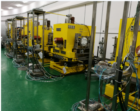
Figure 7: Location retest of secondary collimator absorbers
