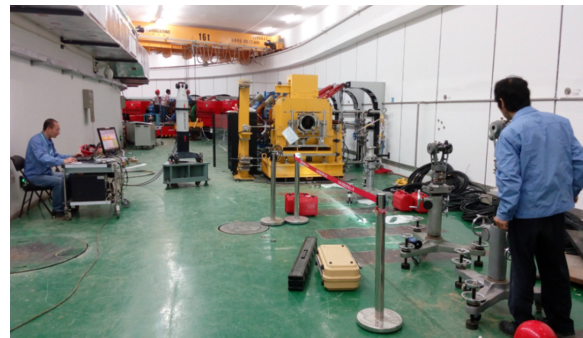
Figure 4: Position calibration of primary collimator scrapers.
