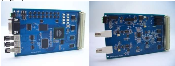
Figure 7: MB & ADC/DAC board of DPSCM.
