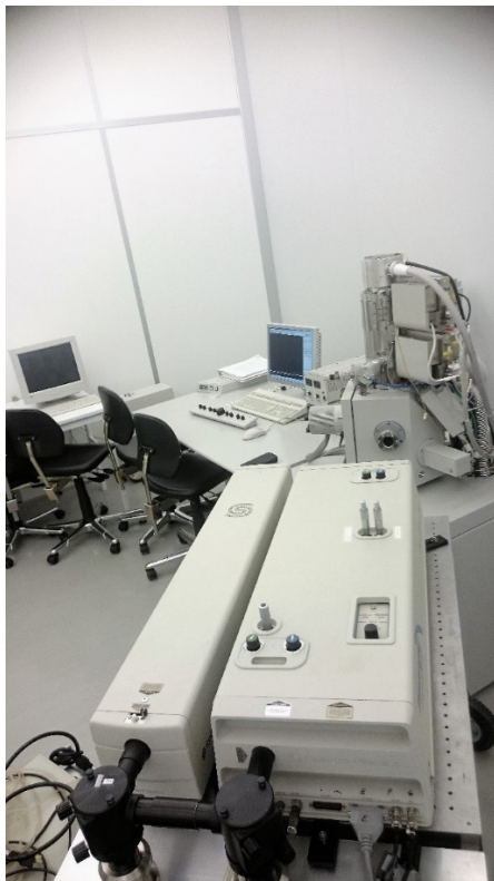
Figure 2: Installation of lasers in front of SEM at the Ångström Laboratory clean room.
