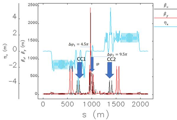
Figure 1: Collision optics of the JLEIC ion ring used in this study. Crab cavities are placed in the inner horizontal CCB locations at each side of the IP, where  $\beta_x$  is high, as indicated by the blue arrows.
