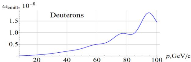
Figure 3: Incoherent part of the deuteron resonance strength in the JLEIC ion collider ring.
