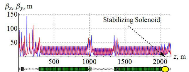
Figure 1:  $\beta$  functions of the ion collider ring.
