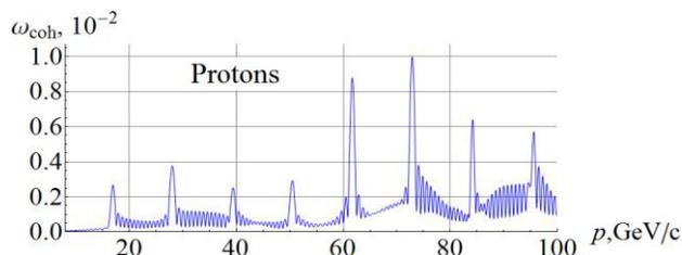
Figure 4: Coherent part of the proton resonance strength in the ion collider ring.
