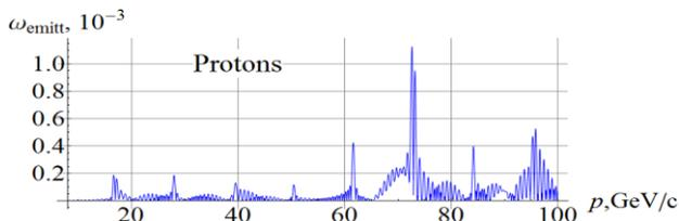
Figure 2: Incoherent part of the proton resonance strength in the JLEIC ion collider ring.
