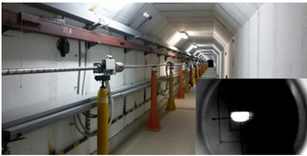
Figure 3: VEPP-5 – VEPP-2000 beam transfer line (right down corner – view of the beam at the phosphor screen at the end of transfer line).
