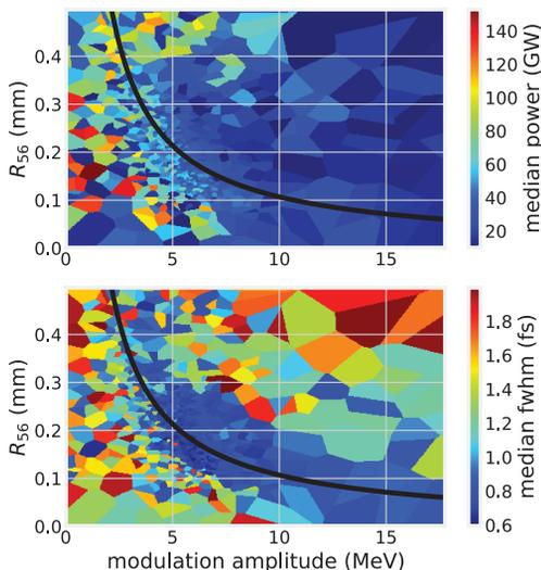
Figure 2: The peak power (top) and fwhm duration (bottom) are shown for a 6 undulator segment optimization. The undulator segment taper was also part of this optimization, though this axis is not shown explicitly. In this plot the non-uniform sampling of the sample space results the optimization algorithm’s search through parameter space. The black line indicates the  $R_{56}$  required to stand the slice up vertically.
