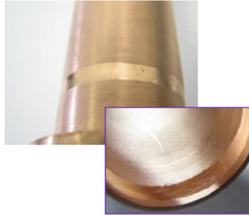
Figure 9: Circumferential weld profile
