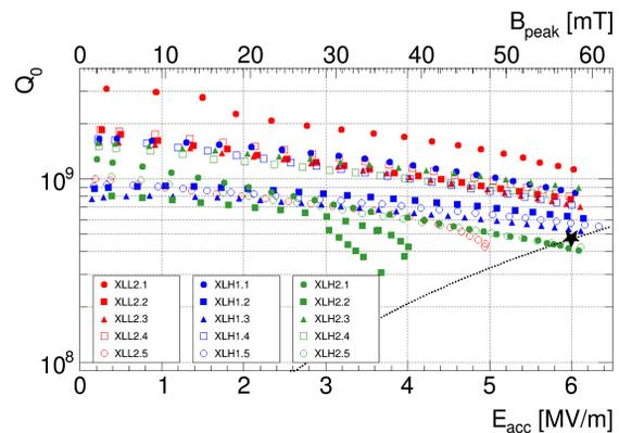
Figure 5:  $Q$  vs  $E_{acc}$  curves of the HIE-ISOLDE linac cavities.
