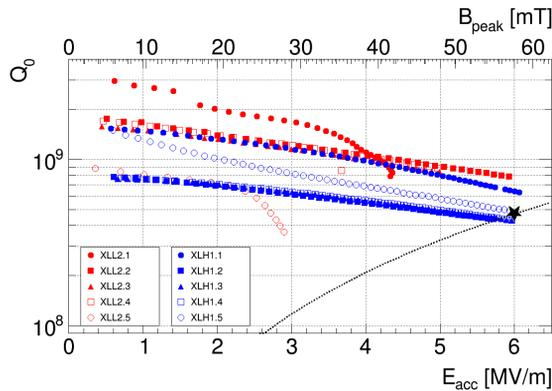
Figure 1: Q vs  $E_{acc}$  curves of diode sputtered cavities, data from July 2016. Label XLL2 refers to CM1 and XLH1 to CM2.
