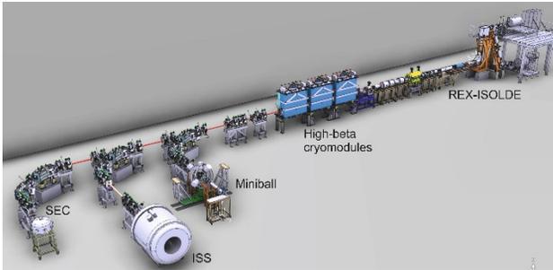
Figure 4: A 3D visual of the HIE-ISOLDE linac, composed of three cryomodules, and the three experimental stations in the HEBT. At the end of the first beam line, XT01, Miniball is located, at the second (XT02) the ISOL Solenoidal Spectrometer, ISS, and the third, XT03, is reserved for movable setups. In the drawing, XT03 is occupied by the Scattering Chamber, SEC [2].
