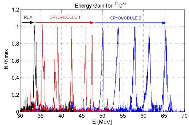
Figure 2:  $^{12}\text{C}^{3+}$  beam energy spectrum for all cavities [2].
