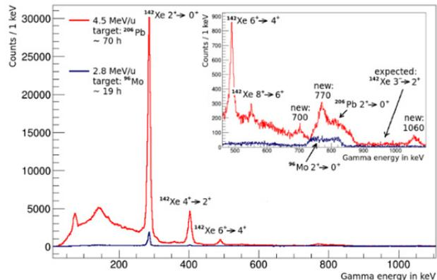
Figure 3: Doppler-corrected gamma ray spectrum of 4.5 MeV/u  $^{142}\text{Xe}$  beam Coulomb excited on  $^{206}\text{Pb}$  target (in red) and the equivalent gamma spectrum for 2.8 MeV/u  $^{142}\text{Xe}$  beam on a  $^{96}\text{Mo}$  target (in blue). The higher energies of HIE-ISOLDE markedly improve the population of higher-lying states (Courtesy of C. Henrich) [6].
