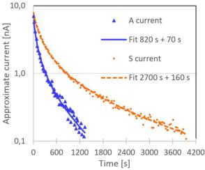
Figure 5: Current of 10 keV  $Xe^+$  in both rings, estimated from the Schottky area for one measurement in each ring. The lines are fits to Eq. (1) with  $1/A_{rg}$  and  $1/A_{i}$  given in the legend.
