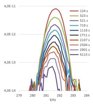
Figure 4: Schottky signal squared vs frequency in ring S. The signal can be followed for more than an hour. 10 keV Xe<sup>+</sup> at the 20<sup>th</sup> harmonic with background subtracted and the injected current is around 7 nA. The numbers in the legend show the average time after injection. With time one sees a slight decrease of the average frequency but very little frequency broadening.
