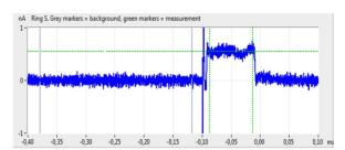
Figure 2: Current vs time in the Faraday cup for a 10 keV C<sub>3</sub> beam averaged over 10 cycles. The current in the dump is measured between the green markers, while zero is defined by the average between the grey markers. At -0.10 ms we see noise from the switch of the injection power supply.
