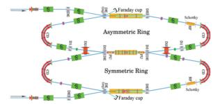
Figure 1: Top view of DESIREE with the positions of Fara- day cups and Schottky detectors indicated. Each ring is 8.6m in circumference.
