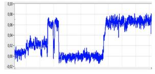
Figure 3: Current of  $10 \text{ keV C}_{60}$  in the beam dump (0-0,07 nA), averaged over 10000 cycles. Each point is the moving average of 20 cycles.
