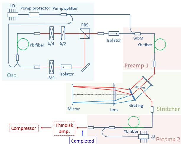
Figure 5: Experimental Setup.
