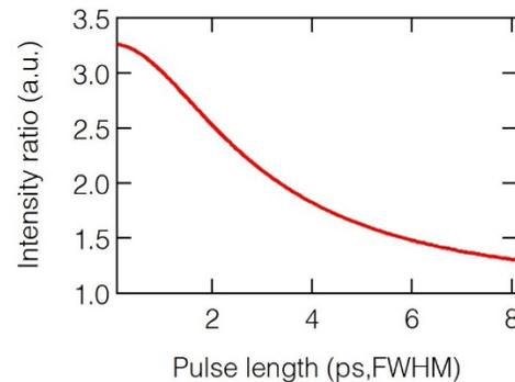
Figure 2: Relationship between Intensity Ratio and Pulse Length.
