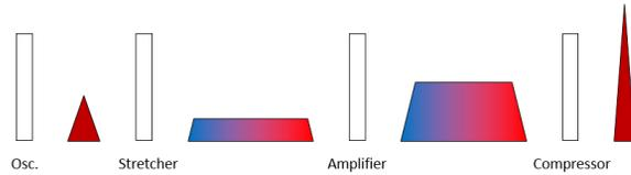
Figure 3: Chirped Pulse Amplification.
