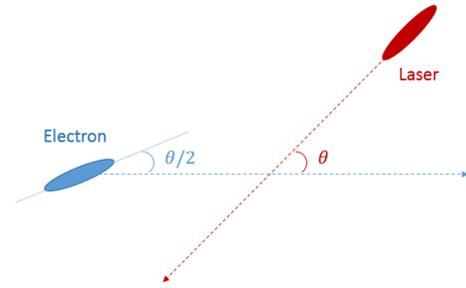
Figure 1: Crab Crossing Laser-Compton Scattering.
