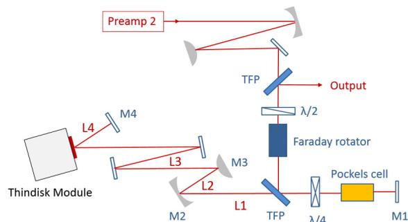
Figure 6: Setup of the thindisk amplifier.
