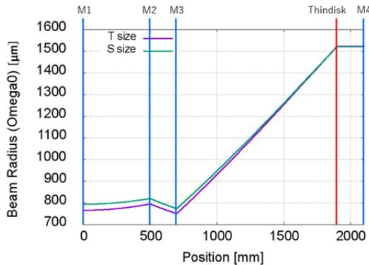
Figure 7: Mode size in the resonator.
