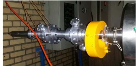
Figure 9: Prebuncher and diagnostic cavities with similar structures in connection with linac beam pipe.
