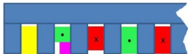
Figure 1: End field configuration at the beginning of the upper coil. In yellow are indicated auxiliary coils 1 (AUX1), in magenta auxiliary coils 2 (AUX2), and in red and green the main coil, wound in opposite direction to create the alternating magnetic field. Similar configurations are at all 3 other ends.
