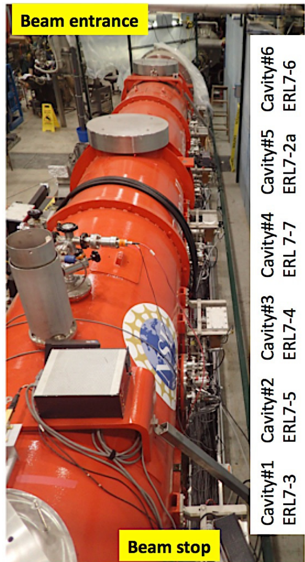
Figure 5: Present commissioning (May 2017) of the MLC.
