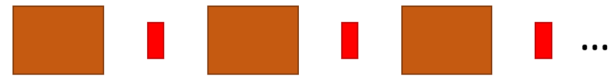
Figure 3: Diagram of the linac optics showing the RF cavities (brown) and the permanent magnet quadrupoles (red).
