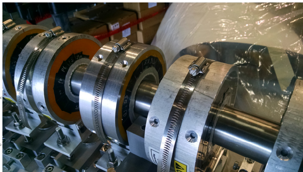
Figure 3: The focusing (in the middle) and the defocusing (left side of the figure) Halbach type magnets.
