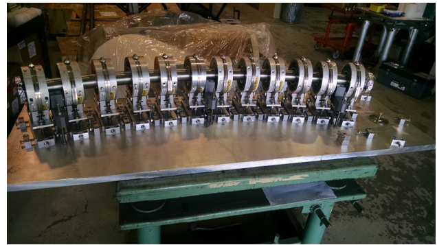
Figure 1: NS-FFAG with 12-magnet girder at BNL.
