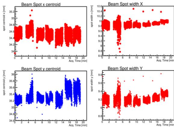
Figure 5: Beam x and y cross section synthetic parameters (centroid and width) corresponding to the same conditions of Fig. 4.
