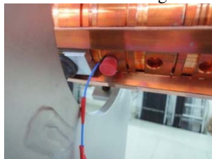
Figure 5: A K-type thermocouple is mounted on the linac section with a red rubber cork.
