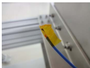
Figure 4: K-type thermocouple with a kapton tape for electrical insulation at low thermal gradients.
