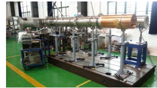
Figure 5: Beam window chambers.
