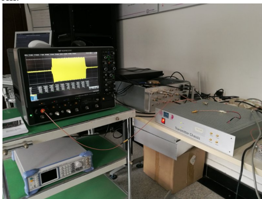
Figure 9: Experiment setup for testing LLRF system
