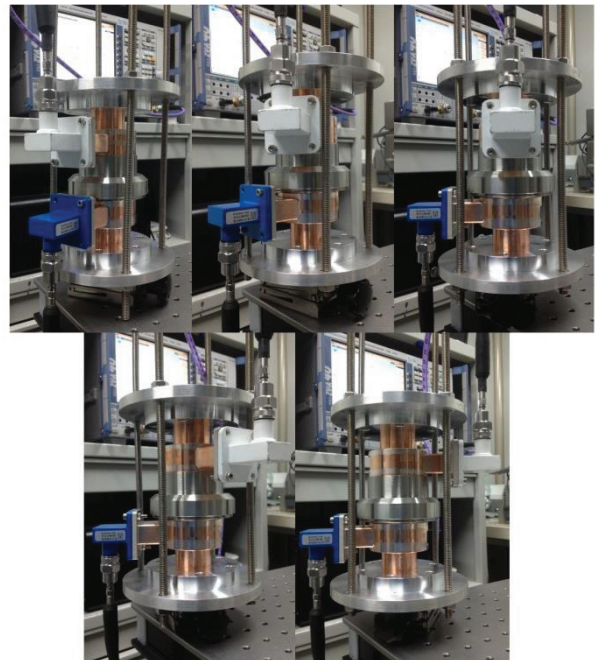
Figure 7: RF measurement setup of the rotary joint.
