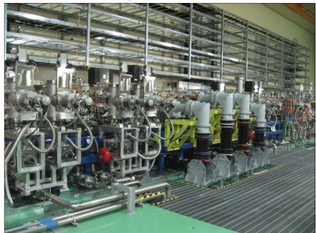
Figure 1: RFQ assembled with high power couplers.
