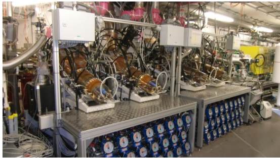
Figure 3: BESSY HOM cavities installed at BESSY II
