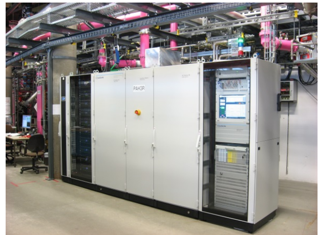
Figure 4: 500 MHz 80 kW CW solid state amplifier.
