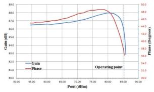
Figure 5: Gain and Phase as a function of Output Power.
