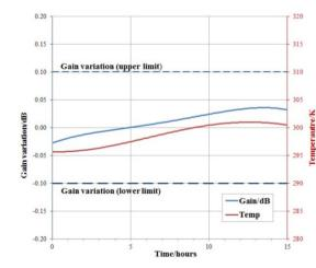
Figure 7: Gain and Ambient Temperature over Time.
