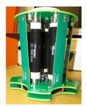
Figure 2: Combiner Balance Resistors with Shielding.
