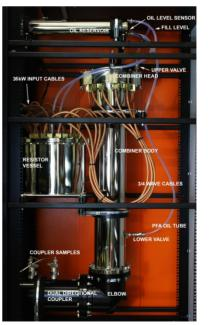
Figure 4: 340 kW Output Combiner.
