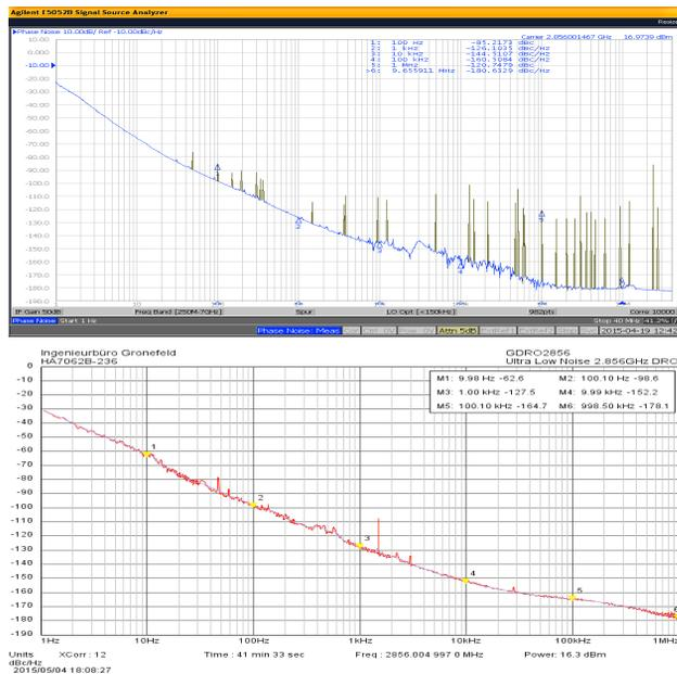
Figure 3: Phase Noise of free-running 2.856GHz DRO.
