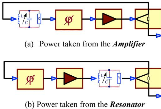
Figure 2: Transmission oscillator.
