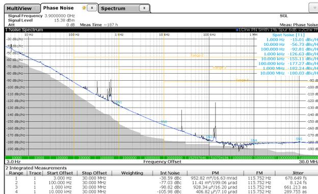
Figure 4: Phase Noise of free-running 3.9GHz DRO.
