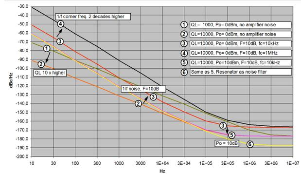
Figure 1: Oscillator PN from (1) with varying parameters.
