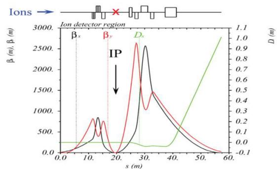
Figure 2: Asymmetric design of the IR optics.
