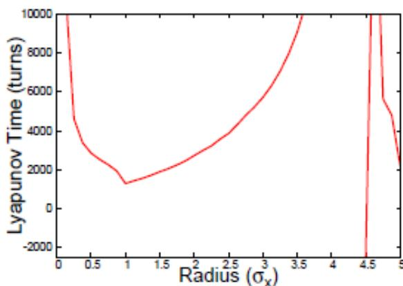
Figure 5: Here we show the Lyapunov time for the system outlined in Table 2. The time goes to infinity at zero since the beam beam effect is treated as a lens in this system and a particle directly on the centreline will feel no kick.
