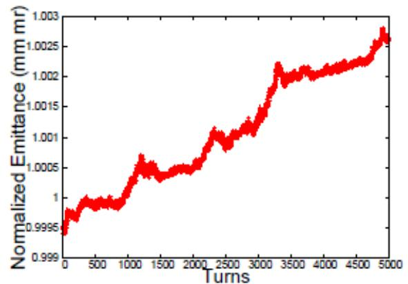
Figure 4: Plot of normalized horizontal emittance in the proton beam over 5000 turns with random  $0.05\sigma$  horizontal jitter. This will model a linac type system.
