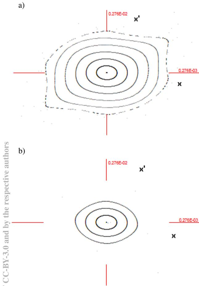
Figure 2: The top, figure 2a) is an example of a horizontal Poincaré section of a beam whose map has been calculated to 4<sup>th</sup> order, while figure 2b) has been
