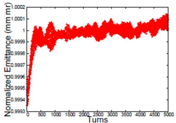
Figure 3: Plot of normalized horizontal emittance in the proton beam over 5000 turns modelled as a synchrotron. The beam begins with an initial  $0.05\sigma$  horizontal offset.
