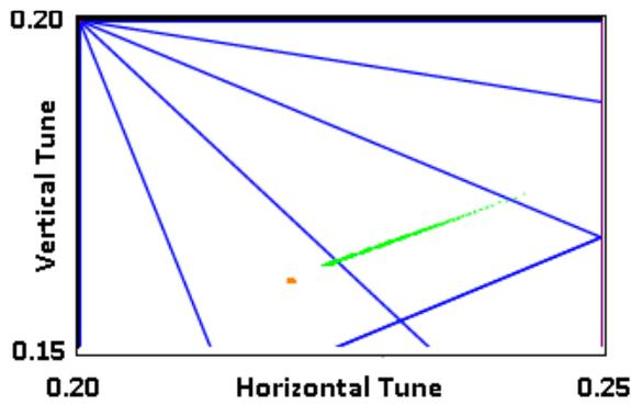
Figure 1:  $4\sigma$  tune footprint of the system. The orange indicates the tune without beam-beam, while the green represents the altered tune.
