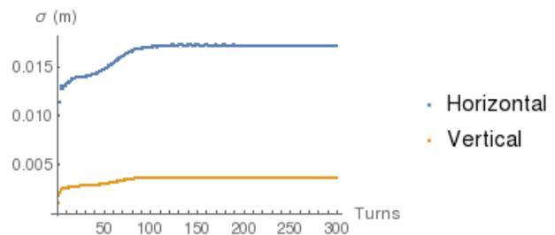
Figure 6: A plot of the beam sizes during the injection phase of the booster ramp cycle
