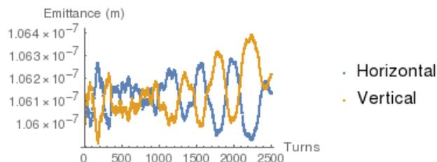
Figure 1: Emittance evolution of the beam at extraction energy. The differences shown are small enough that during the brief period in which the beam is still in the booster, space charge induced emittance growth can be ignored.
