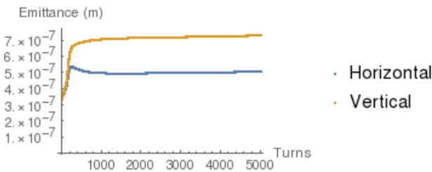
Figure 3: Here we see the emittances of the beam at the cooling pause. The current design calls for electron cooling which is not included in this early simulation, but we can determine an upper limit to the emittance growth of the beam due to space charge.
