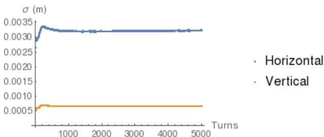
Figure 4: The beam sizes at the injection point of the beam are plotted for the horizontal and vertical dimensions during the cooling phase of the booster cycle.
