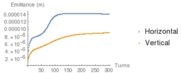
Figure 5: Here we see the evolution of the beam emittances at injection. This is not a complete injection simulation, but shows that even at full charge the emittance growth is not a runaway effect.
