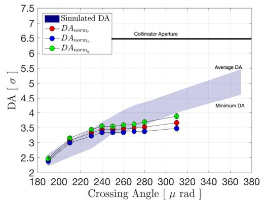
Figure 3: Comparison of tracking simulations to the measured DA for the nominal colliding bunches including measured intensity, emittance and linear coupling from the 2016 LRBB MD.
