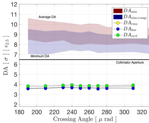
Figure 5: Comparison of simulation and measured DA for the HO only bunch including measured intensity, emittance, and linear coupling.
