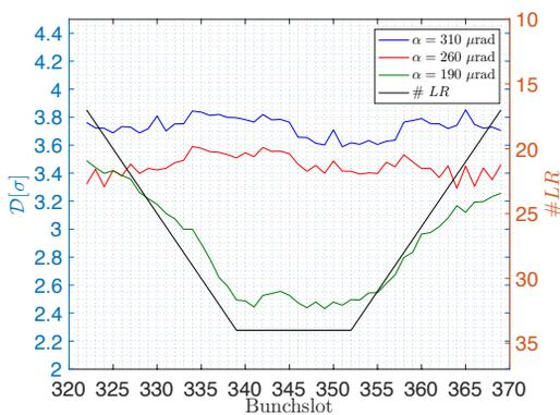
Figure 2: Measured dynamic aperture normalised to  $\epsilon_n = 2.5 \mu\text{m}$  for the first train in the LR beam-beam machine study.
