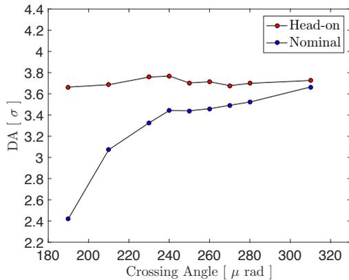
Figure 1: The measured DA from intensity loss normalised to  $\epsilon_n = 2.5 \mu\text{m}$  for the HO colliding bunch and the mean DA for nominal bunches colliding at IP1 and IP5 with both HO and the maximum number of 34 LR beam-beam interactions.
