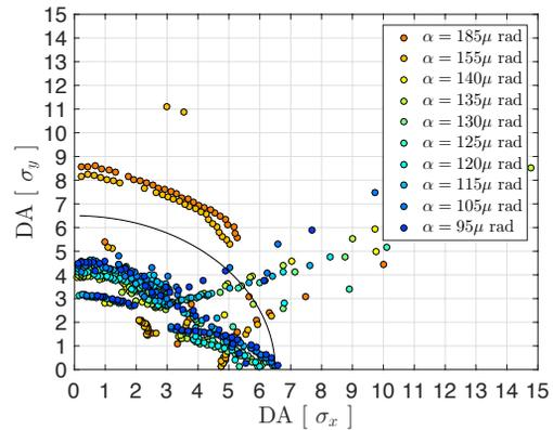
Figure 7: DA from tracking simulations in the  $x - y$  plane including lattice errors, measured intensity, and measured emittance for the HO only colliding bunch. The collimator aperture is shown as the black curve.
