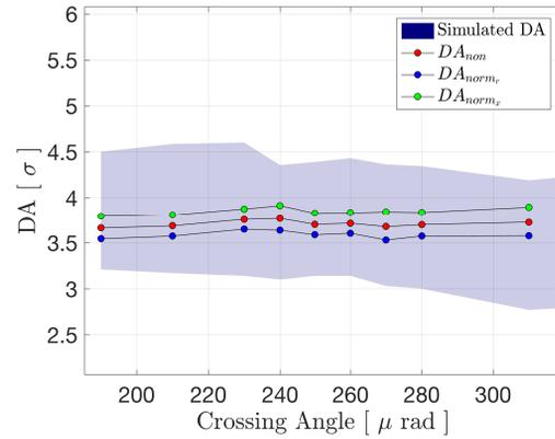
Figure 6: Comparison of tracking simulations to the measured DA for the HO only bunch including measured intensity, emittance and magnetic errors.
