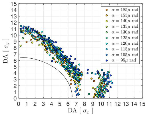
Figure 4: DA from simulations in the  $x - y$  plane including linear coupling, measured intensity and emittance for the HO only colliding bunch. The collimator aperture is shown as the black curve.
