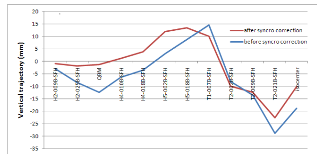
Figure 3: T line measured vertical trajectory before (blue line) and after (red line) synchrotron orbit correction.
