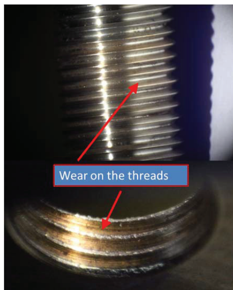
Figure 9: Optical inspection images of the threads of the tuner after the cold test.
