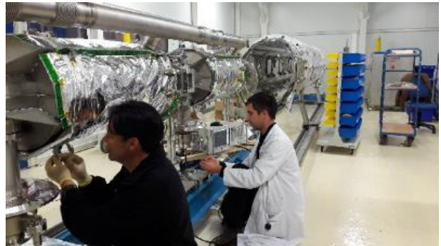
Figure 5: Elliptical cavity cryomodule string assembly.
