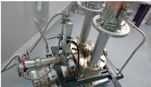
Figure 3: The first pair of power couplers assembled on the RF coupling cavity.
