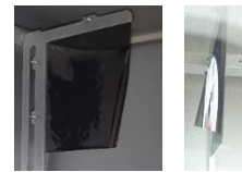
Figure 8: Graphene foils observed to curl in storage.
