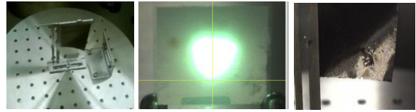
Figure 10: (Left to right) DLC foil mounted in vacuum chamber, 3.6 mm 100 \mu\text{A} electron beam spot focussed on a phosphor screen beneath the foil, observed deformation.
